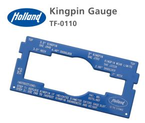
Routine inspection of kingpins is just as important as the inspection of its fifth wheel mating partner. The HOLLAND Kingpin Gauge is a simple and easy to use tool for indicating undersized 2" and 3-1/2" SAE kingpins in need of replacement because of wear. This multi-purpose gauge can be used to check the length and straightness of the kingpin, and check the flatness of the bolster plate. The economical HOLLAND kingpin gauge is readily available from your local dealer or distributor.
