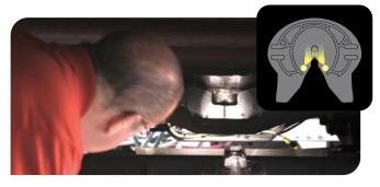
SUCCESSFUL COUPLING - A successful couple triggers highintensity white LED lights, strategically aimed at the kingpin and lock for enhanced visibility during the inspection process, especially in poor weather and low-light conditions.
