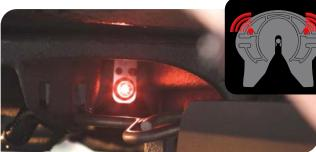
**FAILED COUPLING** – In the case of a failed coupling attempt, bright red flashing LED lights assist the driver to quickly recognize a potentially costly mistake before attempting a tug test or driving away.
