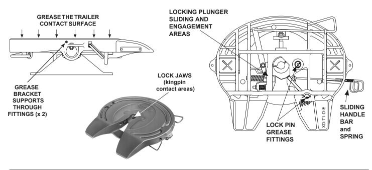
NOTE: Perform the following every three (3) months or 50,000 km, whichever comes first. Thoroughly steam clean all components before inspecting or adjusting.
