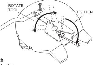
Continue to alternate tightening (clockwise) the adjustment bolt 1/4 turn at a time, until the fifth wheel lock is tight against the kingpin in the lock tester.
