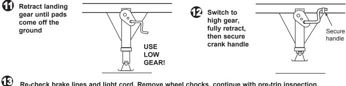
Re-check brake lines and light cord. Remove wheel chocks, continue with pre-trip inspection.
