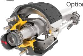
Now available with dressed drum brake configuration, complete your CBX AeroBeam Suspension/Axle system with SAF SC5 wheel ends. Featuring 161/2" x 7" extended life brake linings, industry standard hub, long lasting seals and bearings, and a peace of mind 5-year waranty.
